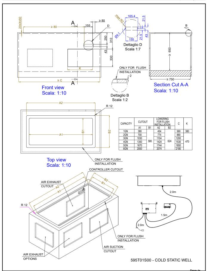
Drop-in refrigerated well, static (1 GN container capacity)
